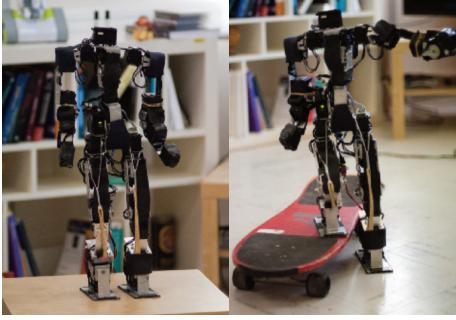
**Passive dynamics inspired from Humans:** when a human walks and moves, he uses gravity as well as the inertia of his body in order to conserve energy. The human walk consists essentially of a fall perpetually caught. The principle is applied to Acroban, as for other recent robots, but extended in this case to the whole body and the torso in particular.
