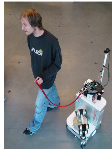
Figure 1: Setup allowing a human to teach paths to a mobile robot. The control architecture is designed learn changes in the robot's own motor dynamics (strong differences in the proprioceptive flow of the wheels). Thanks to a leash, the human can pull on a sensing device, thus guiding the robot. The robotic arms are not used in this study.
