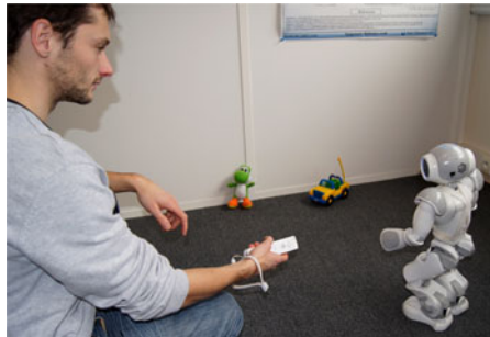
Fig. 7. Users can move the robot by using the directional cross or directly orienting the Wiimote to aim its head. However, the lack of feedback makes it very difficult to estimate whether the robot really sees the object the user wants to teach.
