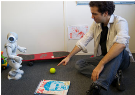
Fig. 11. In this mode of interaction, the robot is guided by the hand and arm gestures made by the user. In order to have a robust recognition, we used a WOZ framework, where the wizard was only seeing the interaction through the robot’s viewpoint.
