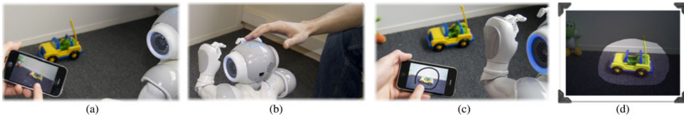
Fig. 3. To make the robot collect a new learning example, users have to first draw the robot's attention toward the object they want to teach through simple gestures. Once the robot sees the object, they touch the head of the robot to trigger the capture. Then, they directly encircle the area of the image that represents the object on the screen. The selected area is then used as the new learning example. (a) Draw the attention toward an object. (b) Trigger the capture. (c) Encircle the area of the object. (d) New learning example.
