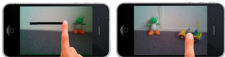
Fig. 5. Drawing attention toward an object: The user first sketches directions to position the robot such that the object is in its field of view (left), and if he wants to center the robot's sight on a specific spot, the user can just tap on the screen (right).
