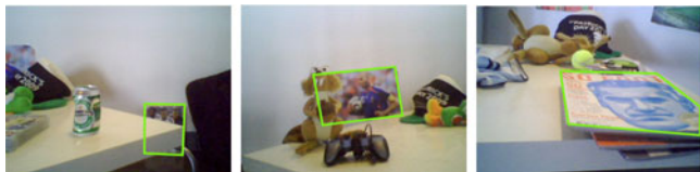
Fig. 22. While the feedback provided by the Laser interface allows users to make sure that the object is visible, it does not help them to realize how the object is actually perceived by the robot. (Left) Video game is almost entirely occluded by the table. (Center) Cluttered foreground in front of the poster of Zidane. (Right) Image of the magazine has been taken with an almost horizontal point of view.
