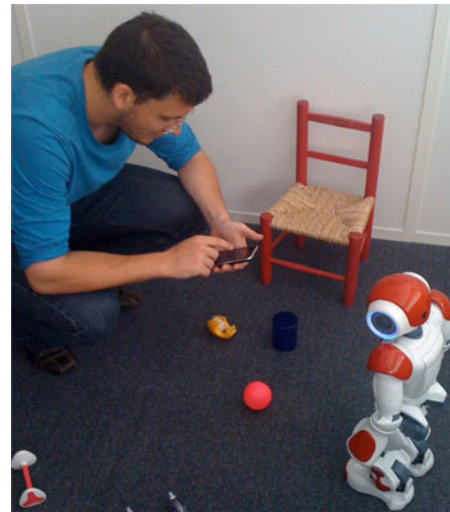
Fig. 1. Using a device as a mediator object between the human and the robot to control the movements of a personal robot allows nonexpert users to teach it how to recognize new visually grounded objects.
