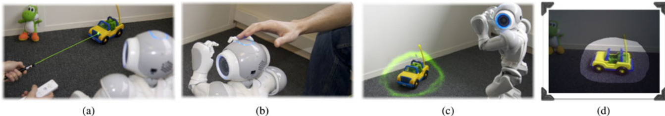
Fig. 9. With this interface, users can draw the robot’s attention with a laser pointer toward an object. The laser spot is automatically tracked by the robot. They can ensure that the robot detects the spot, thanks to the haptic feedback on the Wiimote. Then, they can touch the head of the robot to trigger the capture of a new learning example. Finally, they encircle the object with the laser pointer to delimit its area, which will be defined as the new learning example. (a) Draw the attention toward an object. (b) Trigger the capture. (c) Encircle the area of the object. (d) New learning example.
