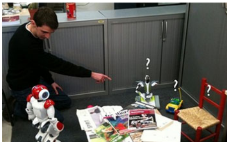
Fig. 2. To allow users to designate a particular object to a robot in a cluttered environment, we need to provide them with a robust and accurate pointing detection. Otherwise, it may lead to restrictive interaction and even to false learning examples.
