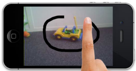
Fig. 6. Once the user asks the robot to take a picture of a new object, he can directly encircle it, thus providing a useful rough object segmentation.
